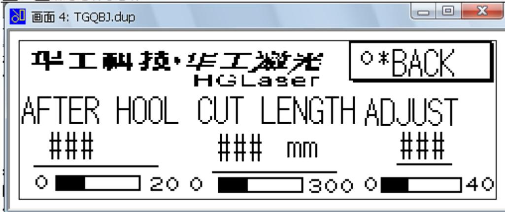
3) "Sensor detect the connect hole and mark times" (AFTER HOLE) setting, this means in the working process when the sensor detect the hole how many paper will continue to mark. Example: when set 0, after detect hole, paper will continue to move and cut, the moving distance set through "CUT LENGTH", if set 2, it means paper will move to mark two papers and then cut.
