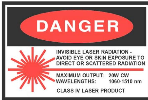
Label of warning      Location:    at the cover or the front panel of the laser
