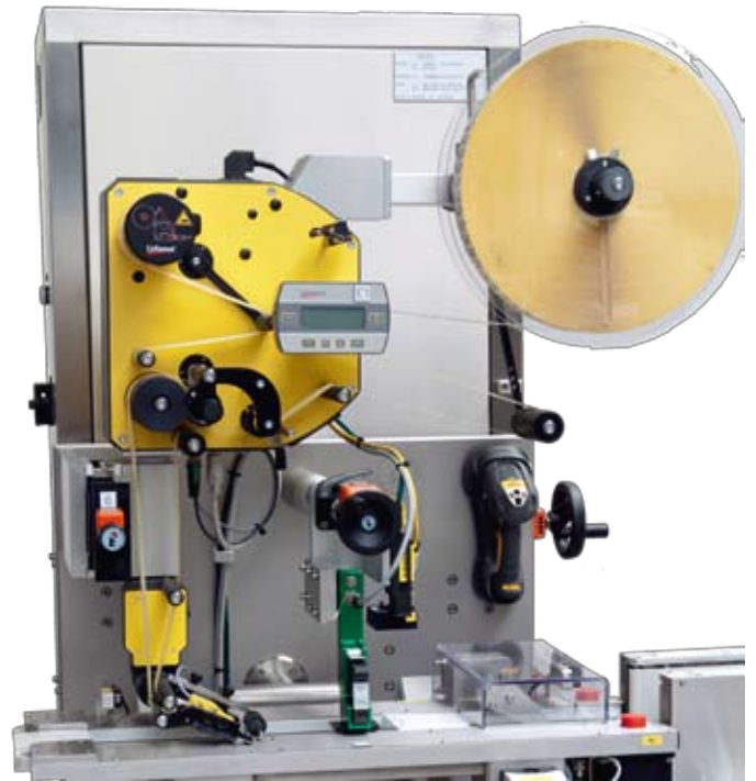
Collamat NG 50 X top labeling and sealing of pharmaceutical products. Nominal capacity 200 products per minute. Max. capacity 100'000 labels per hour
