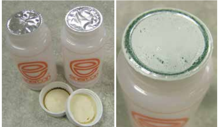
Excessive wrinkling, signs of burning or discoloration on either the liner or in the cap indicates that either the output is set too high or the line speed is too slow.
