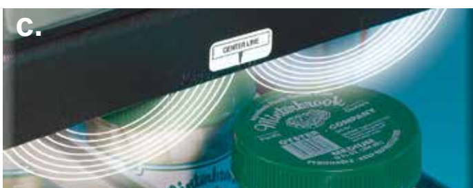
Depending on the cap and container geometry different sealing heads may be required for optimal sealing efficiency. Picture above are common sealing head designs: (a) Tunnel sealing head, (b) Deep tunnel sealing head, (c) Flat sealing head, (d) Original All-in-one sealing head .
