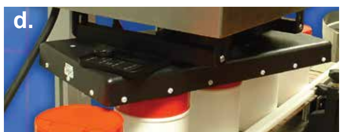
Depending on the cap and container geometry different sealing heads may be required for optimal sealing efficiency. Picture above are common sealing head designs: (a) Tunnel sealing head, (b) Deep tunnel sealing head, (c) Flat sealing head, (d) Original All-in-one sealing head .
