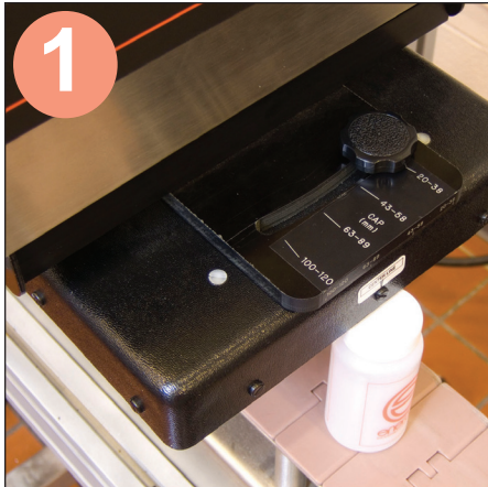
Align the power supply and sealing head over the conveyor with the sealing head in the 20-38mm position.
