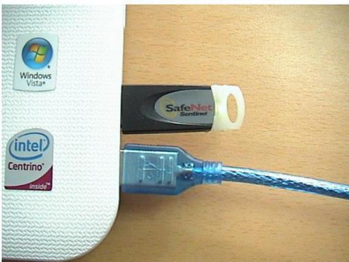
2 Instal key dongle connect USB from computer to laser
