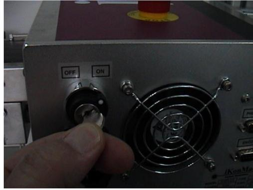
Switch on at power and Key to on
