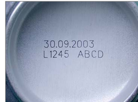
Cans coated with laser-sensitive paint
