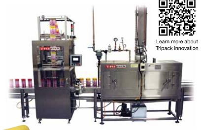
SLEEVE LABELER. In the sleeve labeler, cans of Barbasol's Pure Silk Raspberry Mist shaving cream receive a full-body shrink label for club store twin-packs, then the bundled packs move into the steam tunnel.
