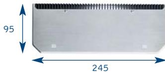
Controller Front Elevation
